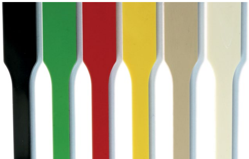
Fig. 14: Coloured AKROTEK® PK tension rods (non-reinforced)
