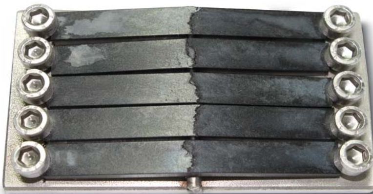
Fig. 7: Significant damage to test specimens made from standard PA6.6-GF30 after just 2 hours immersed in \text{ZnCl}_2 solution
