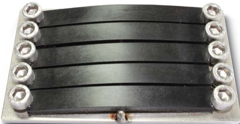
Fig. 8: No material damage of AKROMID® A3 GF 30 1 L black (4436) even after 200 hours immersed in \text{ZnCl}_2 solution
