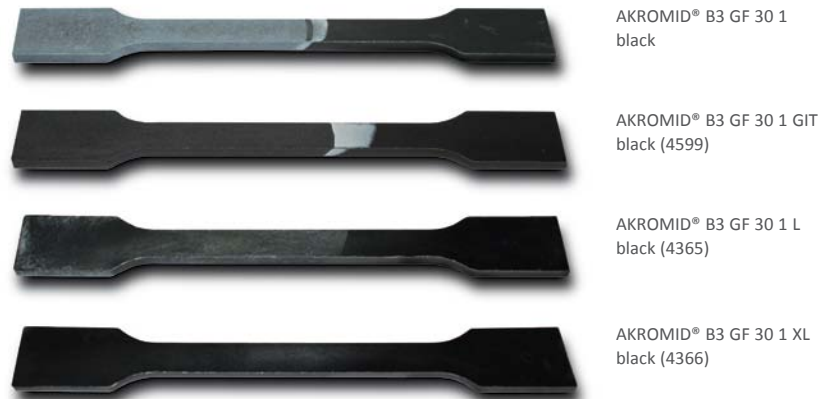
Fig. 6: Tension rods made from various AKROMID® compounds after immersion in \text{CaCl}_2 (in accordance with DBL 5416).
